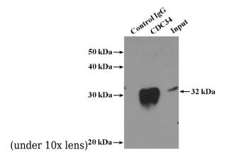
IP Result of anti-CDC34 (IP:Catalog No:109102, 4ug; Detection:Catalog No:109102 1:500) with mouse testis tissue lysate 4000ug.
