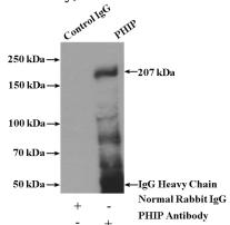
IP Result of anti-PHIP (IP:Catalog No:113817, 4ug; Detection:Catalog No:113817 1:3000) with A375 cells lysate 3600ug.
