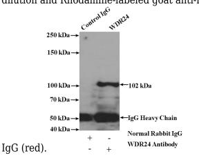
IP Result of anti-WDR24 (IP:Catalog No:116861, 4ug; Detection:Catalog No:116861 1:500) with HeLa cells lysate 3200ug.
