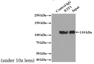
IP Result of anti-RTF1 (IP:Catalog No:114858, 4ug; Detection:Catalog No:114858 1:500) with
