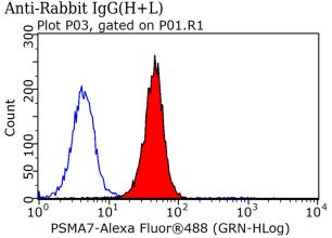
1X10^6 HepG2 cells were stained with 0.2ug PSMA7 antibody (Catalog No:114377, red) and control antibody (blue). Fixed with 90% MeOH blocked with 3% BSA (30 min). Alexa Fluor 488-congugated AffiniPure Goat Anti-Rabbit IgG(H+L) with dilution 1:1500.
