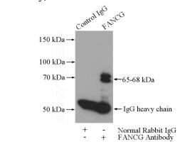
IP Result of anti-FANCG (IP:Catalog No:110519, 4ug; Detection:Catalog No:110519 1:300) with mouse testis tissue lysate 4000ug.
