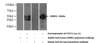
Transfected HEK-293 cells were subjected to SDS PAGE followed by western blot with Catalog No:110063(DPEP2 Antibody) at dilution of 1:1000
